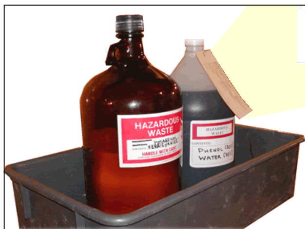
Example of Secondary Containment
